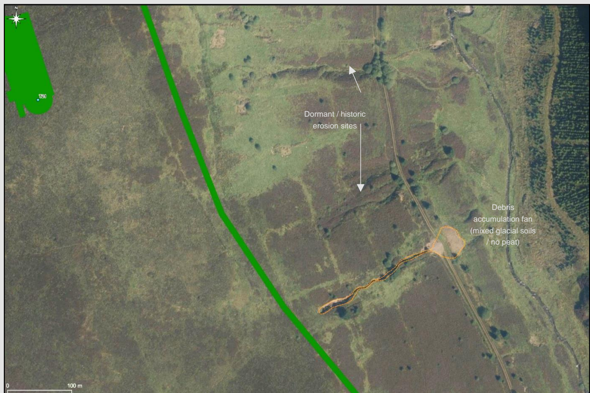
Figure: Extract from Geomorphological Mapping Showing previous mass movement (superficial soils) type location south-east of T21.
