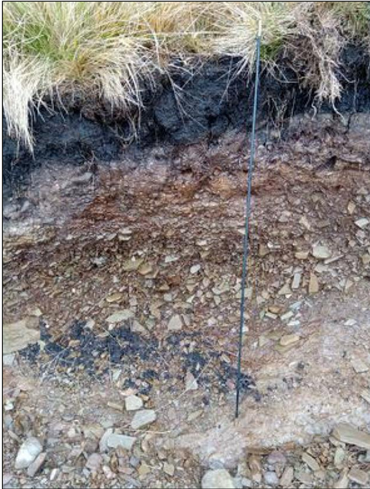
Figure 9.7: Example soil profile at Turbine T32 showing thin peat layer (1m probe for scale)
